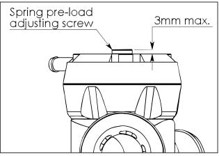
Take the car for a drive, and note how easily the valve vents when you lift off. Making the spring softer will allow the valve to open easier and vent longer, and increasing the pre-load means you will need to drive the car harder (i.e. more boost) before you start to hear the valve venting, and the blow-off sound will be shorter in duration.
